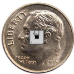
The small size of germicidal UV LED chips allows for easy integration with devices. RayVio, a leading manufacturer of UV LED products, has designed a UV LED chip for germicidal purpose that's smaller than a quarter. The tiny chip can easily be integrated with medical equipment, bathtubs, doorknobs, and even mobile devices.
